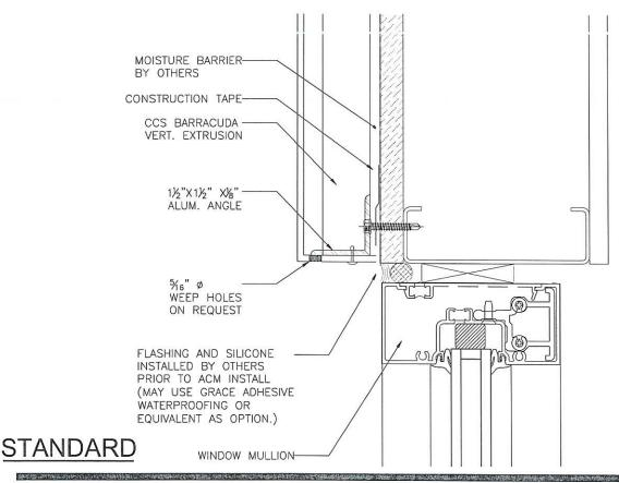
1/2"±×3" MOISTURE CONSTRUCTION SUPPORT BARRIER TAPE WITH BLOCKING AS SILICONE (BY CCS) REQUIRED FOR (BY OTHERS) WINDOWS TBD BY PLYWOOD OR SHEATHING CCS (BY OTHERS) BARRACUDA FRAMING **EXTRUSION** (BY OTHERS) ACM PANEL-(BY CCS) LINE SHEET ROCK OF (BY OTHERS) T-TRIM CCS ALUM. WINDOW SINTRA BOARD **EXTRUSION** BARRIER (BY CCS) ALUMINUM POP RIVET (BY CCS) FILL CAVITY MANO MATO WITH WINDOW **EXPANDING** MULLION FOAM (BY OTHERS) SEALANT
